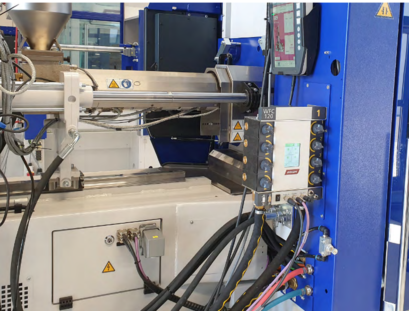
Installation of the WFC 120 close to the mold on a WITTMANN BATTENFELD injection molding machine.
